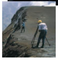
**Figure 1.13** Some volcanoes bulge outward slightly when the pressure from rising molten rock inside them builds up. Before an earthquake, stress builds up causing the ground to tilt slightly. These signs, although not visible to the naked eye, can be detected using a **surveyor's level**, a device that measures minute changes in the angle of the ground's slope.
