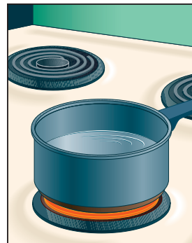
Figure 2.28a) Heat from the hot element reaches the water particles at the bottom of the pot by conduction.
