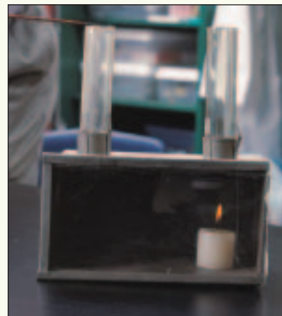
Figure 2.29 Set-up of smoke box
