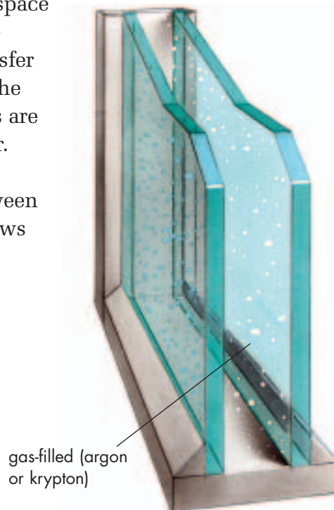
Figure 2.31 An energy efficient window
