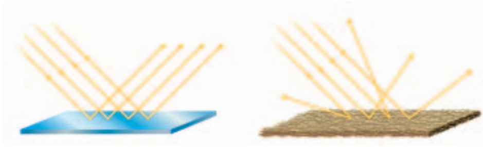
Figure 2.8 Regular reflection (left) and diffuse reflection (right)
